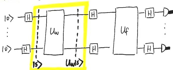
$U_w |w\rangle = -|w\rangle$  and  $U_w |x\rangle = |x\rangle$  for  $x \neq w$
